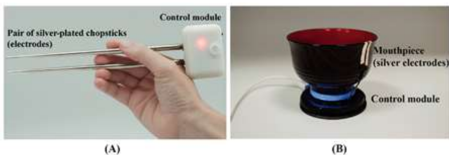
Fig. 1. Prototypes of the two electric taste utensils - (A) pair of chopsticks and (B) soup bowl.
